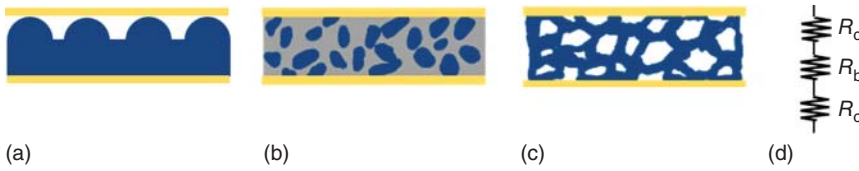
Figure 13.3 Schematics of three representative types of RTS. (a) Microstructured contact. (b) Bulk conductive nanocomposites. (c) Porous conductive materials. (d) A simple equivalent circuit of RTS.
