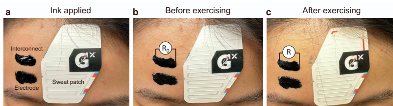
Figure. S15: Photos of the ink sweat stability test, showing the ink trace and sweat pad on the subject's forehead.
