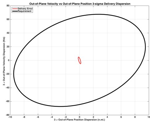
Figure 17. The Trans-Earth Entry Interface Conditions Mapped Crossrange Position vs Crossrange Velocity Delivery Error Ellipses
