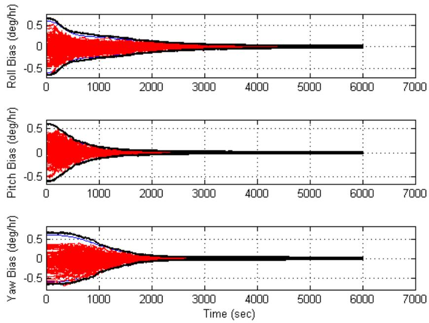
**Figure 2. Gyro bias estimation error of qEKF**
