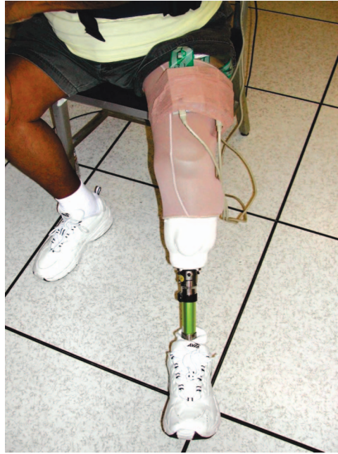
Figure 7. Compliant socket instrumented with Tekscan sensors.
