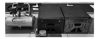
Fig. 2 Main components of the perturbation platform system: two platform units and a tethered, hand-held, remote-control unit (front). High pressure air source located in adjacent room with air line under floor.
