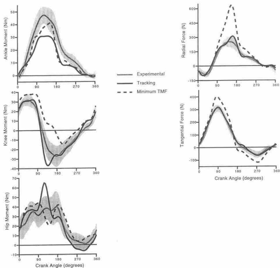
**Figure 1** — Joint moments (extensor  $> 0$ ), tangential pedal forces (perpendicular to crank, propulsive  $> 0$ ), and radial pedal forces (parallel to crank, compressive  $< 0$ ) for experimental data (shading equals  $\pm 2$  standard deviations), optimal tracking simulation, and minimum TMF simulation. Crank angle zero reference is top-dead-center.
