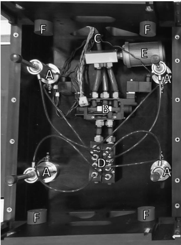
**Fig. 3 Internal view of a single platform. (A) Four pneumatic pistons, (B) 5/3 control valve, (C) high-pressure inlet line, (D) distribution blocks, (E) exhaust muffler, and (F) bump stops to arrest the platform at specific drop heights and angles.**
