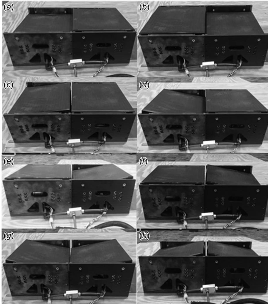
**Fig. 5** Different configurations available. (a) Vertical drop left, (b) vertical drop right, (c) inversion left, (d) eversion left, (e) eversion right, (f) inversion right, (g) eversion bilateral, and (h) inversion bilateral. Not pictured but available are bilateral up, and vertical drop bilateral.
