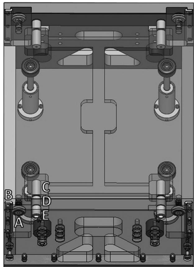
**Fig. 4 Perturbation Platform System design drawing with platform motion control components revealed. Individual components (same for all four corners): (A) V-groove track roller, (B) V-groove rail, (C) sealed linear solenoid, (D) platform brass insert for solenoid mount and pin support, and (E) end plate brass insert for pin support.**
