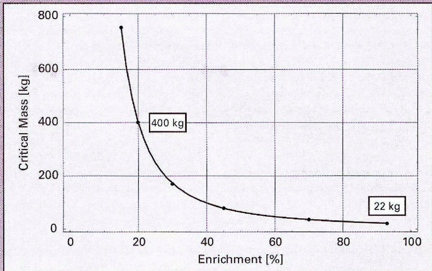
Figure 1 Critical mass of a uranium sphere surrounded by a 5-cm beryllium "neutron reflector" as a function of uranium-235 enrichment.
