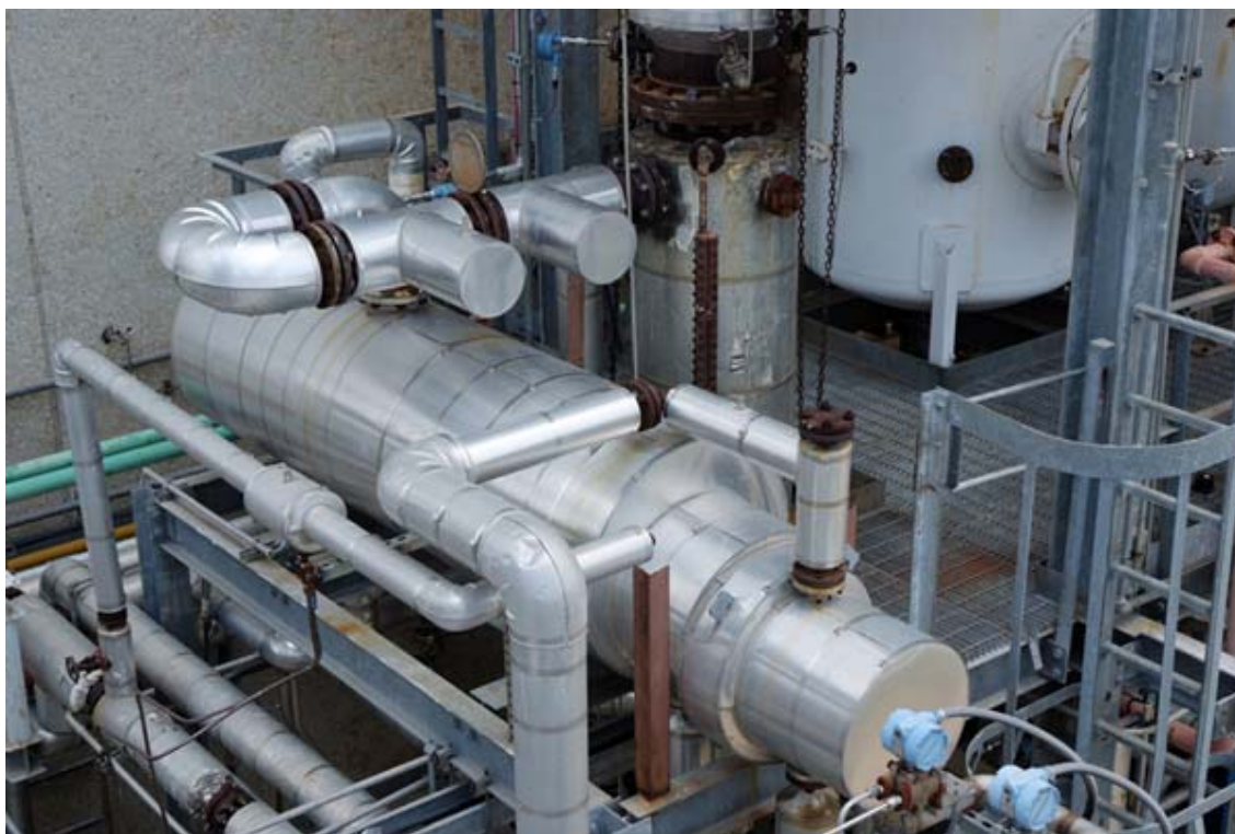
Figure 2-24. Stainless Reboiler and Stripper Column Sump with Calcium Silicate Insulation
