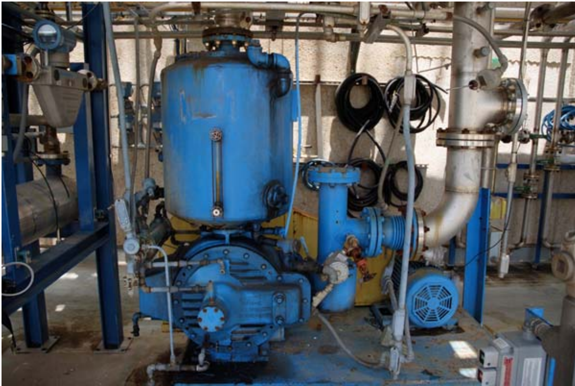
Figure 2-5. Vacuum Pump (C-102A) Draws Gas from the Right Side and Discharges from the Top of the Oil Reservoir (Picture Taken by C. Lewis)
