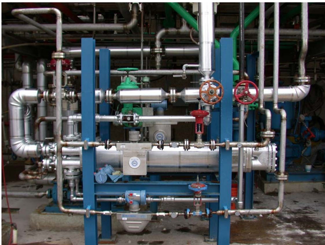
Figure 2-6. Solvent Preheater (H-101A & B), Micro Motion® Flowmeters, and Control Valves Installed on Support Rack (Picture Taken by C. Lewis)
