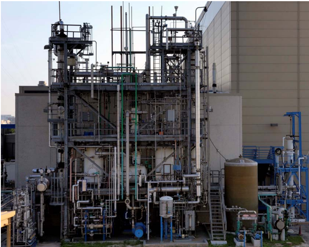
Figure 2-1. Pilot Plant Facility at UT SRP with the Stripper Column and Reboiler on the Left Side, Absorber Column on the Right Side, Absorber Feed Tank and Overhead Gas Accumulator on the First Platform (Picture Taken by C. Lewis)
