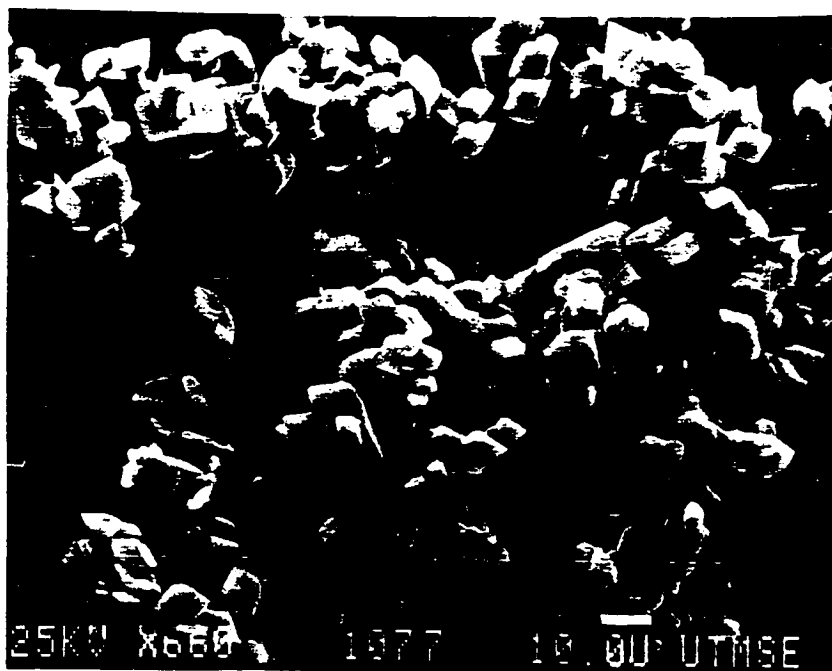
Figure 3.15: Reagent 1 in 6.5 mM \text{SO}_3 , 10% Dissolved Exp 77A - pH 5.3, 0.1M \text{CaCl}_2 , 0.85 atm \text{CO}_2 , 55°C
