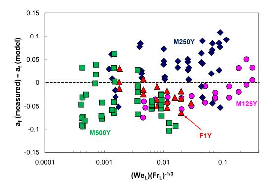
Figure 6.9. Area residuals of M125Y ( $a_p = 125 \text{ m}^2/\text{m}^3$ ), M250Y ( $a_p = 250 \text{ m}^2/\text{m}^3$ ), F1Y ( $a_p = 410 \text{ m}^2/\text{m}^3$ ), and M500Y ( $a_p = 500 \text{ m}^2/\text{m}^3$ ) as a function of ( $We_L$ )( $Fr_L$ )<sup>-1/3</sup>, with  $a_f$  (model) values from equation 6.13.
