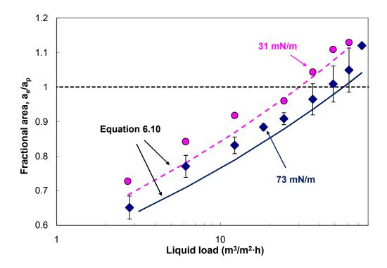
Figure 6.14. Mass transfer area of M250Y ( $a_p = 250 \text{ m}^2/\text{m}^3$ ) at baseline and low surface tension. Error bars denote one standard deviation.
