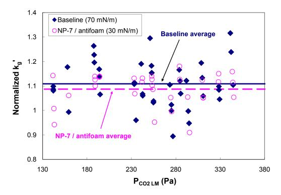
Figure 5.5. Normalized  $k_g'$  of base case (0.1 mol/L NaOH) and surfactant system (0.1 mol/L NaOH + 125 ppm<sub>v</sub> TERGITOL NP-7 + 50 mg/L Q2-3183A antifoam).
