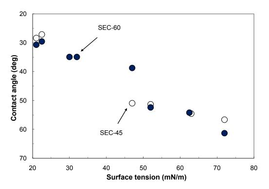
Figure 6.13. Contact angle and surface tension data for two shallow embossed, corrugated ("SEC"), stainless steel surfaces (45° and 60°), reproduced from Nicolaiewsky and Fair (1999).
