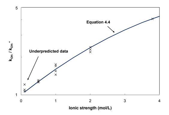
Figure 5.4. Kinetic measurements of CO<sub>2</sub>-NaOH system at 20°C, reproduced from Pohorecki and Moniuk (1988).
