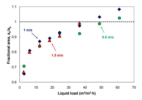
Figure 6.1. Mass transfer area of Mellapak 250Y ( $a_p = 250 \text{ m}^2/\text{m}^3$ ).
