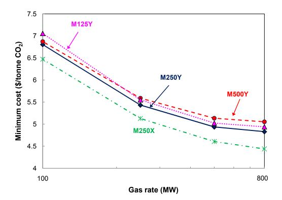
Figure 8.2. Minimum calculated absorber costs for M125Y, M250Y, M500Y, and M250X.
