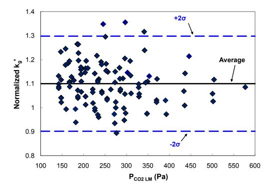
Figure 5.1. Normalized  $k_{g}'$  of base case (0.1 mol/L NaOH) as a function of CO<sub>2</sub> partial pressure.
