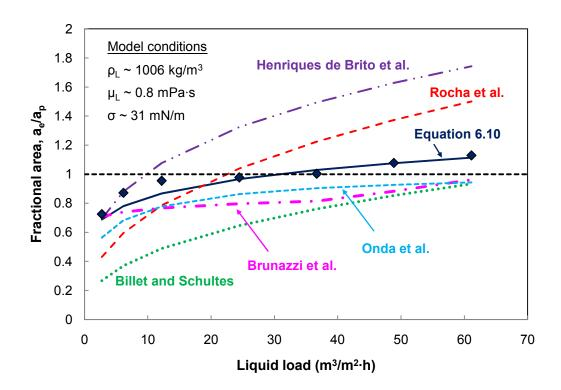
Figure 6.26. Mass transfer area of M250Y ( $a_p = 250 \text{ m}^2/\text{m}^3$ ) compared with predicted values from models at low surface tension.
