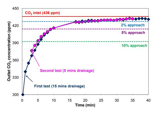
Figure 6.2. Pre-wetting film saturation data obtained with Mellapak 2Y ( $a_p = 205 \text{ m}^2/\text{m}^3$ ). Inlet CO<sub>2</sub> concentration was periodically confirmed, as reflected by gaps in the data (e.g., from 10 to 15 min).
