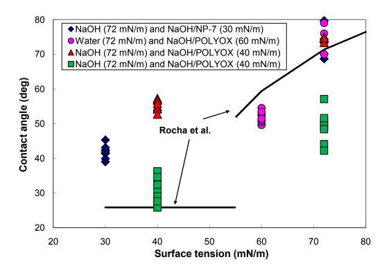
Figure 6.12. Contact angles on stainless steel surface.
