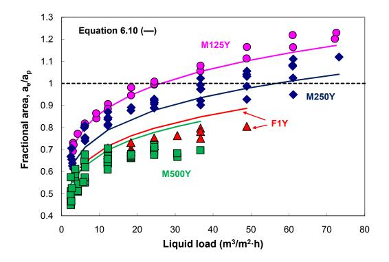
Figure 6.6. Mass transfer area of M125Y ( $a_p = 125 \text{ m}^2/\text{m}^3$ ), M250Y ( $a_p = 250 \text{ m}^2/\text{m}^3$ ), F1Y ( $a_p = 410 \text{ m}^2/\text{m}^3$ ), and M500Y ( $a_p = 500 \text{ m}^2/\text{m}^3$ ).
