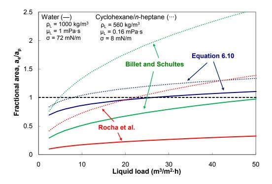
Figure 6.31. Predicted mass transfer area of M125Y ( $a_p = 125 \text{ m}^2/\text{m}^3$ ) from various models. Lines denote water (—) or cyclohexane/*n*-heptane system at 414 kPa (…).
