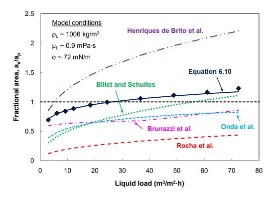
Figure 6.25. Mass transfer area of M125Y ( $a_p = 125 \text{ m}^2/\text{m}^3$ ) compared with predicted values from models.
