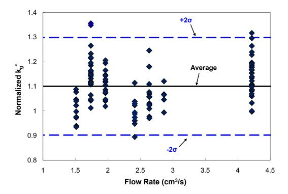
Figure 5.2. Normalized  $k_{g}'$  of base case (0.1 mol/L NaOH) as a function of liquid flow rate.
