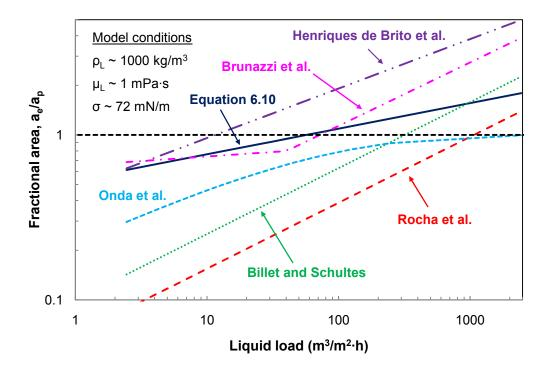
Figure 6.28. Mass transfer area of M250Y ( $a_p = 250 \text{ m}^2/\text{m}^3$ ) compared with predicted values from models, extrapolating out to infinite liquid load limit.
