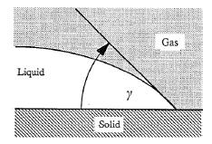
Figure 6.11. Illustration of the contact angle. Slightly modified version of image from McGlamery (1988).
