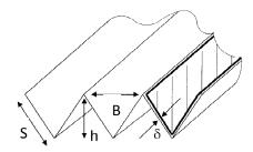
Figure 3.2. Packing channel dimensions. Slightly modified version of image from Olujic et al. (1999).
