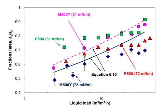
Figure 6.15. Mass transfer area of M500Y and P500 ( $a_p = 500 \text{ m}^2/\text{m}^3$ ) at baseline and low surface tension. Error bars denote one standard deviation.
