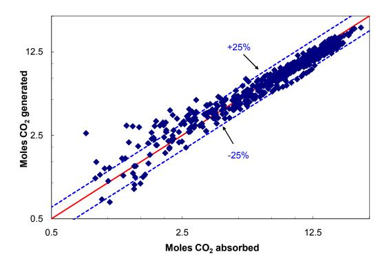
Figure 6.4. CO<sub>2</sub> material balance for packed column experiment.
