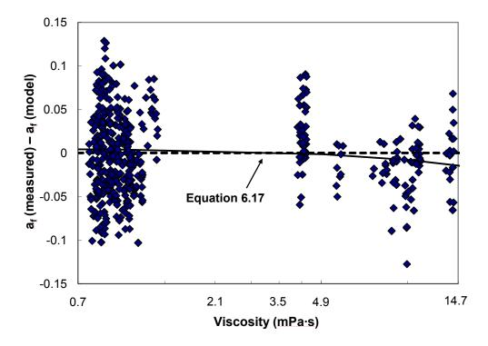
Figure 6.20. Area residuals of experimental database as a function of liquid viscosity, with  $a_f$  (model) values from equation 6.13.
