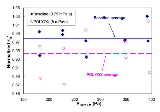
Figure 5.6. Normalized  $k_g'$  of base case (0.1 mol/L NaOH) and polymer system (0.1 mol/L NaOH + 1.25 wt % POLYOX WSR N750).
