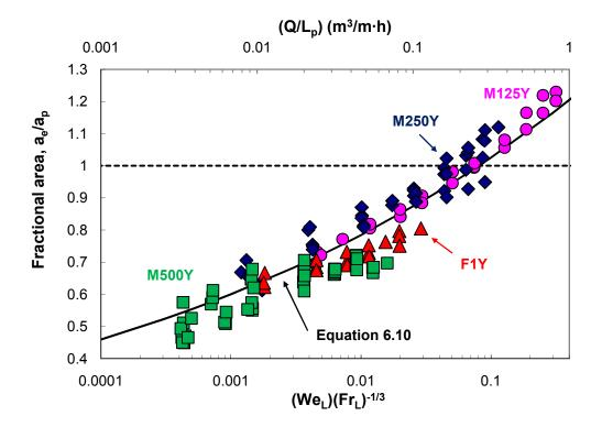
Figure 6.7. Representation of mass transfer area of M125Y ( $a_p = 125 \text{ m}^2/\text{m}^3$ ), M250Y ( $a_p = 250 \text{ m}^2/\text{m}^3$ ), F1Y ( $a_p = 410 \text{ m}^2/\text{m}^3$ ), and M500Y ( $a_p = 500 \text{ m}^2/\text{m}^3$ ) on dimensionless basis (bottom axis) and as a function of flow rate per wetted perimeter (top axis).
