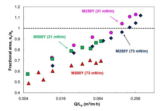
Figure 6.18. Mass transfer area of M250Y ( $a_p = 250 \text{ m}^2/\text{m}^3$ ) and M500Y ( $a_p = 500 \text{ m}^2/\text{m}^3$ ) at baseline and low surface tension as a function of flow rate per wetted perimeter.
