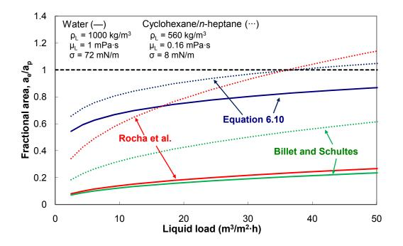
Figure 6.30. Predicted mass transfer area of M500Y ( $a_p = 500 \text{ m}^2/\text{m}^3$ ) from various models. Lines denote water (—) or cyclohexane/*n*-heptane system at 414 kPa (…).
