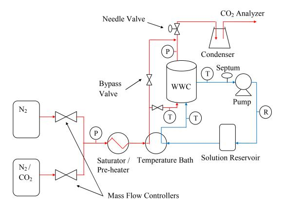
Figure 4.2. Schematic of WWC system. P: pressure gauge, T: thermocouple, R: rotameter.
