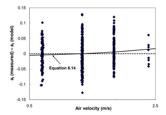
Figure 6.10. Area residuals of experimental database as a function of superficial air velocity, with  $a_f$  (model) values from equation 6.13.
