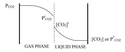
Figure 2.1. Illustration of concentration profiles for CO<sub>2</sub> absorption into liquid.
