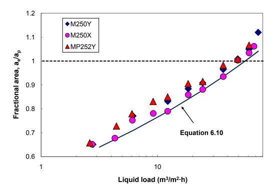
Figure 6.21. Mass transfer area of M250Y, M250X, and MP252Y ( $a_p = 250 \text{ m}^2/\text{m}^3$ ).
