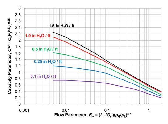
Figure 3.3. GPDC chart for structured packing.
