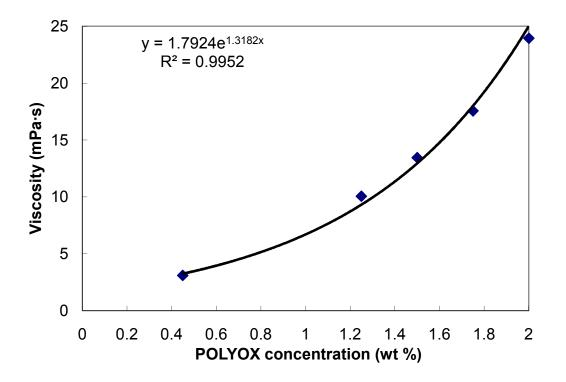
Figure 4.7. Correlation of POLYOX WSR N750 weight percent with solution viscosity at 25°C.
