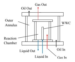
Figure 4.2 illustrates the entire experimental set up. The system was constructed using 1/4-in OD stainless steel tubing and Swagelok<sup>®</sup> fittings. A cloth fiber wrapping was used to insulate the tubing. Gas was supplied from both a N<sub>2</sub> Dewar and a cylinder
