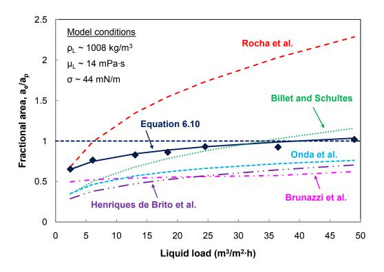
Figure 6.27. Mass transfer area of M250Y ( $a_p = 250 \text{ m}^2/\text{m}^3$ ) compared with predicted values from models at high viscosity.
