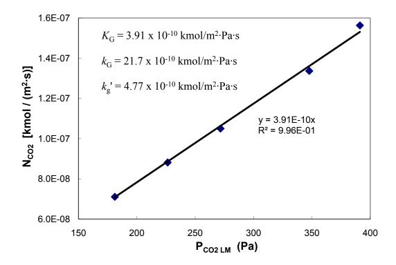
Figure 4.3. Determination of  $k_g'$  using slope method for  $K_G$  (0.1 mol/L NaOH, 32°C).
