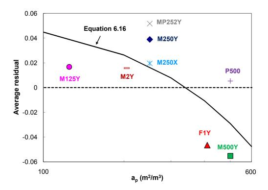
Figure 6.16. Average area residuals of packings at high surface tension as a function of packing size, with  $a_f$  (model) values calculated from equation 6.10.
