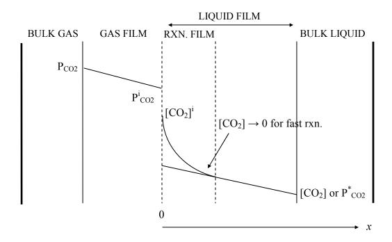
Figure 2.3. Film representation of absorption of CO<sub>2</sub> into liquid with chemical reaction.
