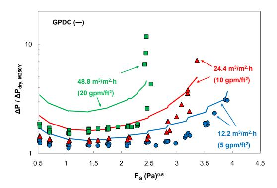
Figure 7.40. Normalized pressure drop of M250Y at liquid loads of 12.2, 24.4, and 48.8 m<sup>3</sup>/m<sup>2</sup>·h (5, 10, and 20 gpm/ft<sup>2</sup>) compared with GPDC.
