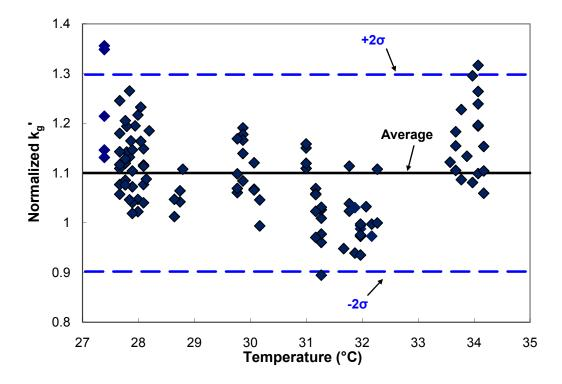
Figure 5.3. Normalized  $k_g'$  of base case (0.1 mol/L NaOH) as a function of temperature.
