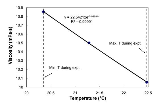
Figure 4.8. Correlation of viscosity with temperature for SRP experiment 0908.
