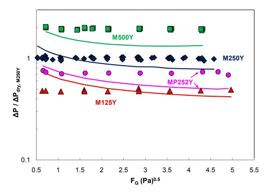
Figure 7.39. Normalized dry pressure drop of M125Y, M250Y, M500Y, and MP252Y compared with GPDC.
