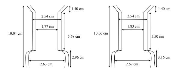
Figure 4.4. "Old" (left) and current (right) WWC reaction chamber dimensions.
