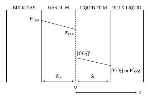
Figure 2.2. Film representation of physical absorption of CO<sub>2</sub> into liquid.
