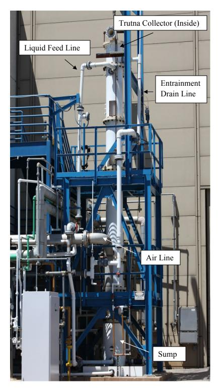
Figure 4.5. Photograph of packed column apparatus.
