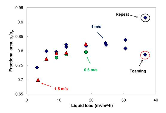
Figure 6.19. Mass transfer area of P500 ( $a_p = 500 \text{ m}^2/\text{m}^3$ ) at low surface tension.
