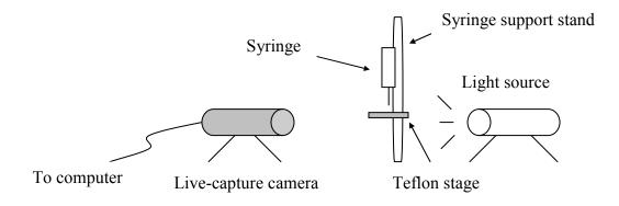
Figure 4.9. Schematic of goniometer set-up.
