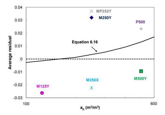
Figure 6.17. Average area residuals of packings at low surface tension as a function of packing size, with  $a_f$  (model) values calculated from equation 6.10.
