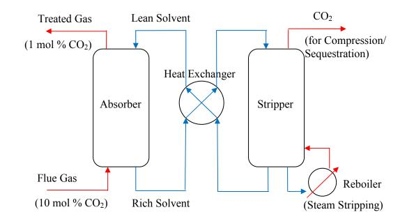
Figure 1.3. Process flow diagram for a CO<sub>2</sub> absorption/stripping process.
