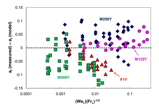
Figure 6.8. Area residuals of M125Y ( $a_p = 125 \text{ m}^2/\text{m}^3$ ), M250Y ( $a_p = 250 \text{ m}^2/\text{m}^3$ ), F1Y ( $a_p = 410 \text{ m}^2/\text{m}^3$ ), and M500Y ( $a_p = 500 \text{ m}^2/\text{m}^3$ ) as a function of ( $We_L$ )( $Fr_L$ )<sup>-1/3</sup>, with  $a_f$  (model) values from equation 6.10.
