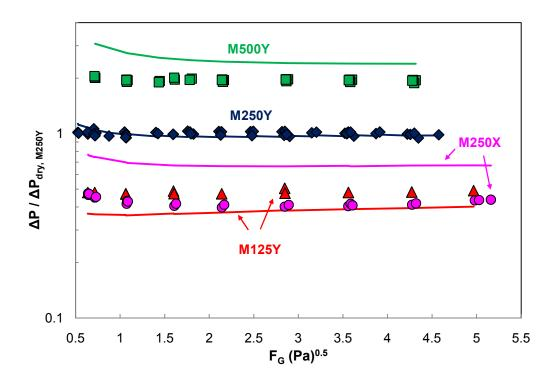
Figure 7.30. Normalized dry pressure drop of M125Y, M250Y, M500Y, and M250X compared with model of Rocha et al. (1993).
