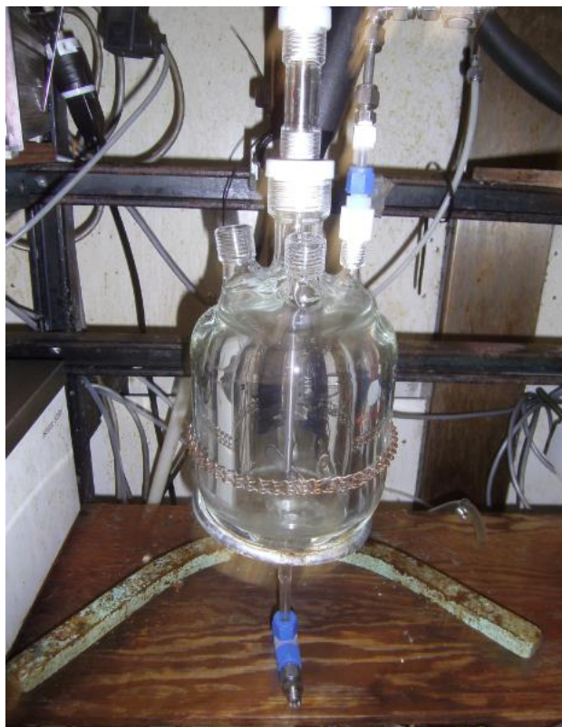
Figure B.3: Jacketed 1000 mL Glass Reactor used for VLE Experiments
