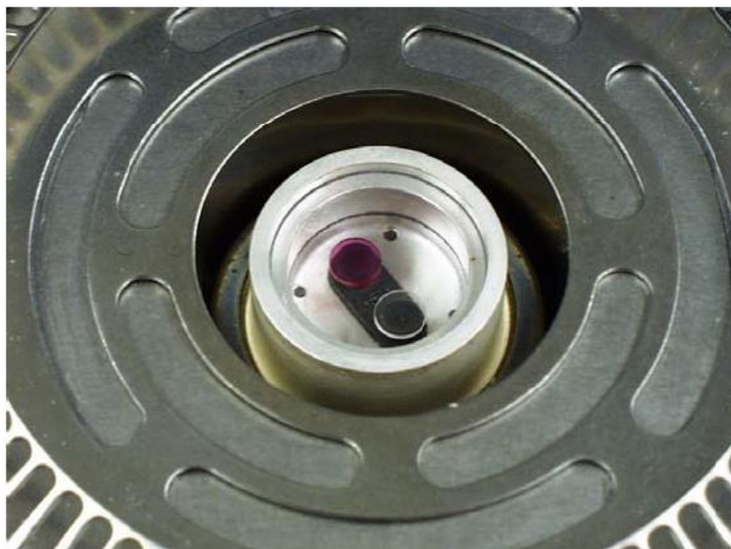
Figure C.1. Snapshot of DSC Internal Chamber: Left (Reference Cell); Right (Sample Cell)
