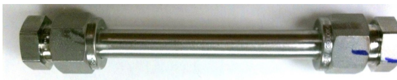
Figure 2.18: Stainless steel thermal cylinder for measuring high temperature nitrosamine formation and decomposition kinetics
