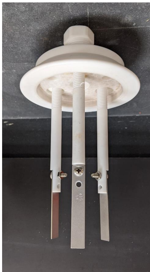
Figure 3-4: Teflon lid with three coupon holders
