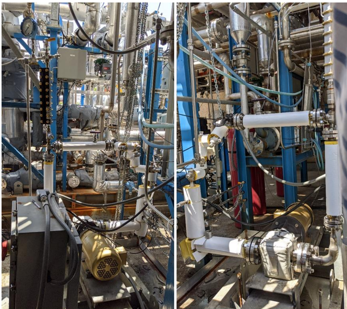
Figure 3-6: Front view (left) and back view (right) of the pump-around corrosion loop.
