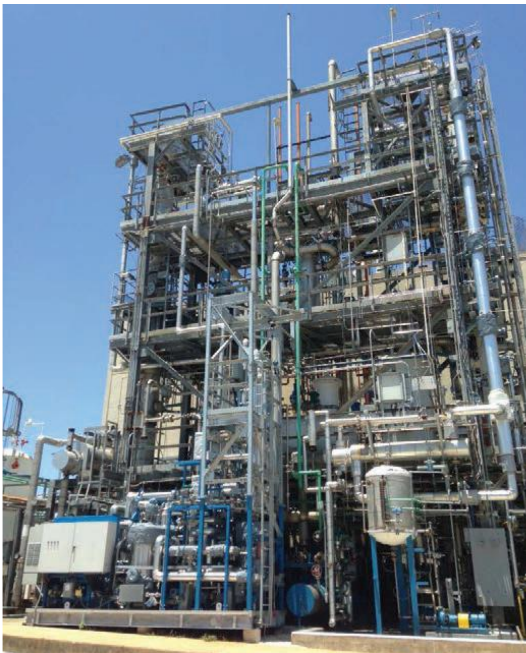
Figure 5-31: SRP pilot absorber/stripper and advanced flash stripper skid (bottom left) (Chen et al., 2017)
