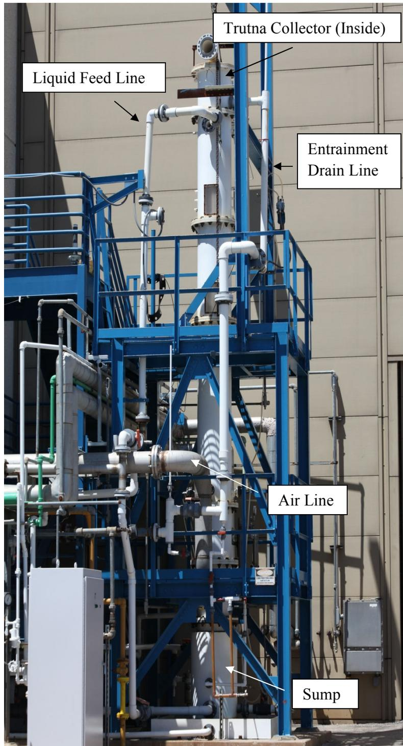
**Figure 4.5. Photograph of packed column apparatus.**
