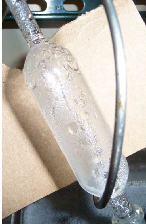
Figure 4: Fogging Test at 150 °C, 7.3–7.7 bar
