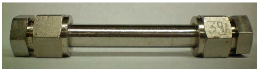
Figure 3.23: Thermal cylinder with “A” end and cylinder number (39) labeled
