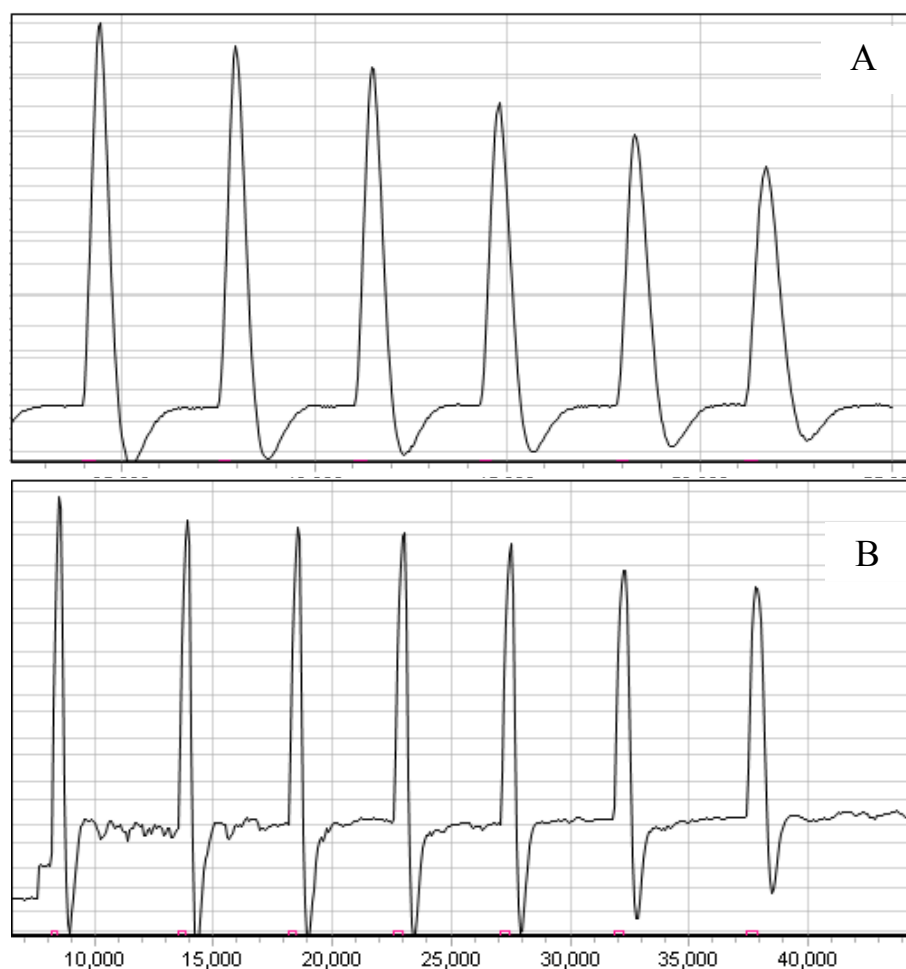
Figure F.12: Comparison of total power baselines for \Delta H_{\text{abs}} measurements at 60 °C (panel A) and 120 °C (panel B)
