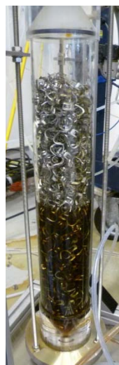
Figure 20: Dumped packing used to eliminate bubbles in the absorber sump
