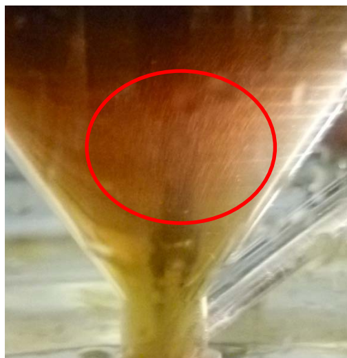
Figure 19: Presence of entrained bubbles in the absorber sump
