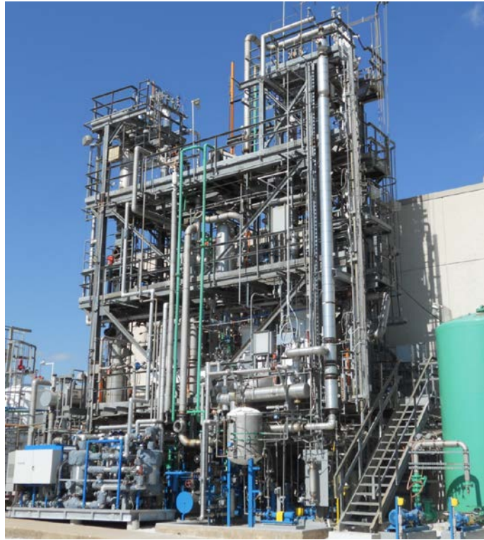
Fig. 3. SRP pilot absorber/stripper system with high temperature flash skid (bottom left).
