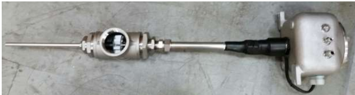
Figure 6: Paddle wheel fan sampler and FTIR probe
