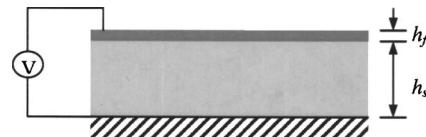
FIG. 1. Schematic of a conductive thin film on a dielectric substrate.
