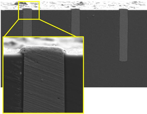
FIG. 4. (Color online) SEM images showing TSV extrusion after thermal cycling.
