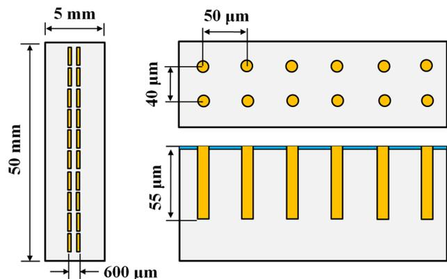
FIG. 1. (Color online) Illustration of the TSV specimen for bending beam tests.
