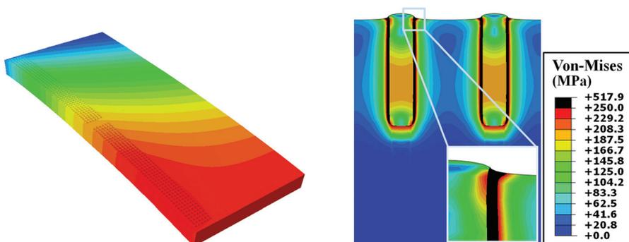
FIG. 5. (Color) FEA results with a thermal load  $\Delta T = 200^\circ\text{C}$ . Left: bending of the TSV specimen (quarter model); Right: plastic deformation and stress distribution.
