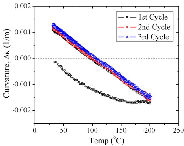
FIG. 2. (Color online) Measurement of curvature difference between a TSV specimen and a reference specimen during thermal cycling.
