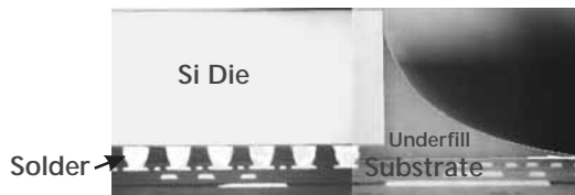
Figure 2.4 Optical micrograph for the package cross-section used for moiré interferometry study.
