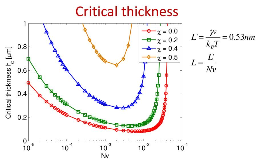
➤ The critical thickness is linearly proportional to L, with the proportionality depending on Nv and X.
