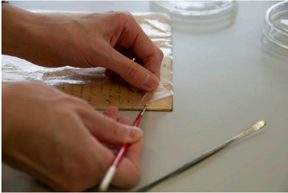
Removing lamination with ethyl acetate
