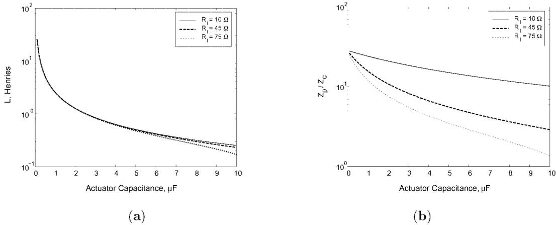
Figure 7. Required inductance and  $Z_p/Z_c$  for  $f = 100$  Hz.
