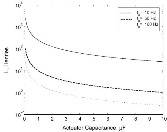
Figure 5. Inductance requirement,  $R_c = R_l$ .
