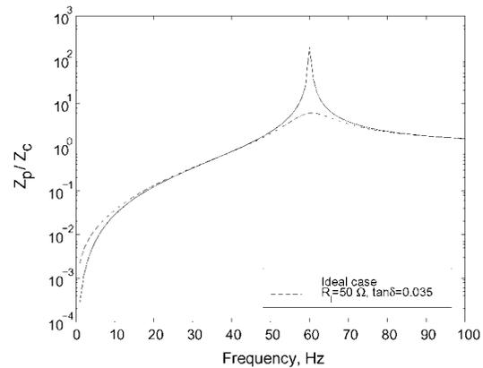
Figure 8. Variation of  $Z_p/Z_c$  with frequency for a  $7 \mu\text{F}$  actuator.
