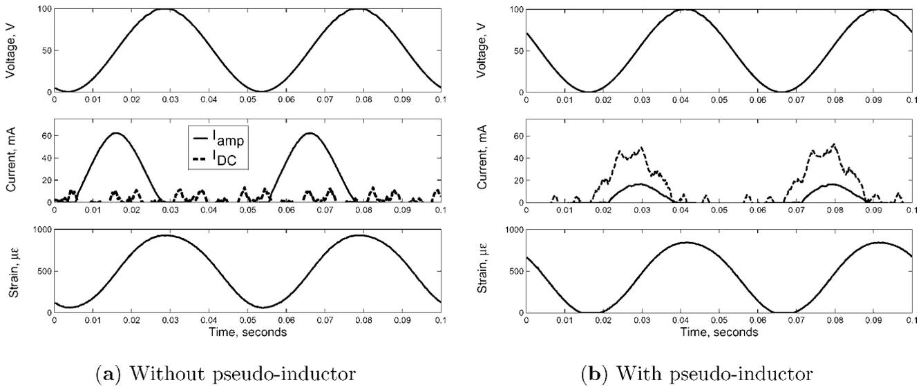
Figure 16. Time variation of voltage, current and strain at 30 Hz.
