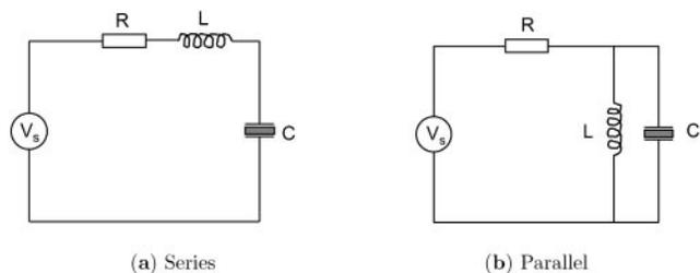
**Figure 1.** Ideal series and parallel configurations.
