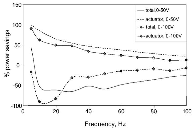
Figure 14. Pseudo-inductor circuit performance with adaptive tuning.
