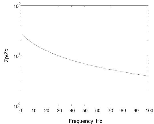
Figure 9.  $Z_p/Z_c$  achievable by continuous tuning,  $7 \mu\text{F}$  actuator,  $R_l = 50 \Omega$ .
