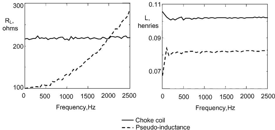
Figure 12. Comparison of choke coil and pseudo-inductor performance.
