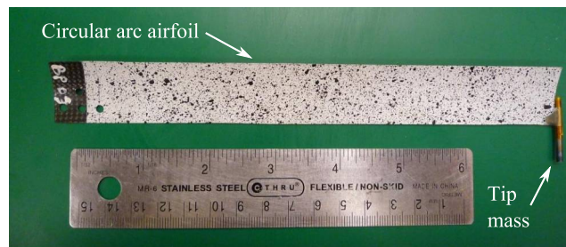
Fig. 4 High-contrast random pattern on the bottom surface of flexible rotor blade.
