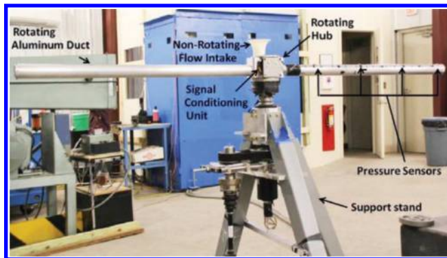
Fig. 1 Duct test article mounted on rotor test stand.
