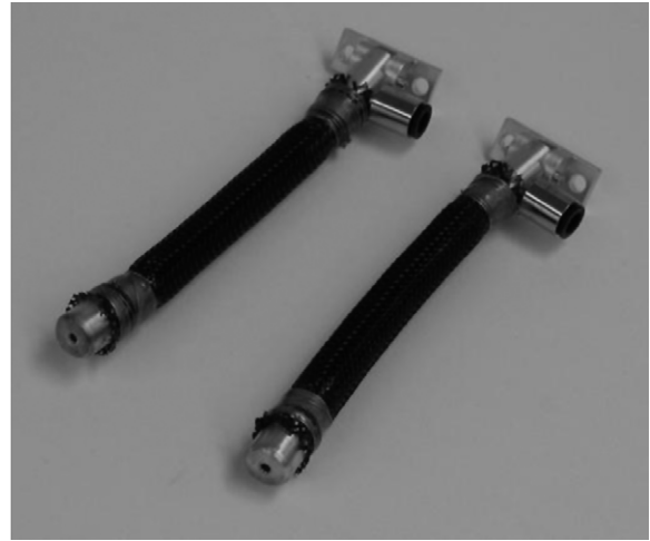
Figure 4. PAMs fabricated for the wind tunnel test article.
