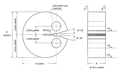
Note 1—All surfaces shall be perpendicular and parallel as applicable within  $0.002\ W$  TIR.
