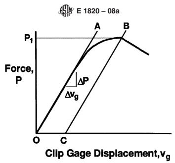
FIG. A4.3 Determination of Initial Compliance
