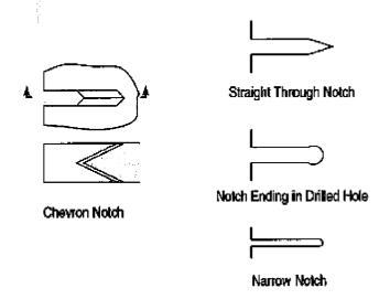
FIG. 6 Fatigue Crack Starter Notch Configurations
