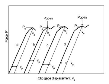
Note 1—Construction lines drawn parallel to the elastic loading slope to give  $\nu_p$ , the plastic component of total displacement,  $\nu_g$ . Note 2—In curves b and d, the behavior after pop-in is a function of machine/specimen compliance, instrument response, etc.
