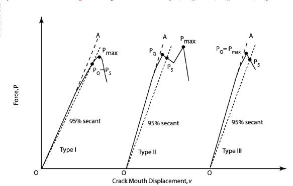
FIG. A5.1 Principal Types of Force-Displacement Records
