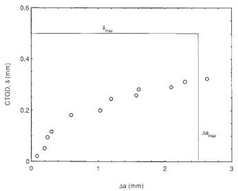
FIG. A10.1 Typical δ-R Curve
