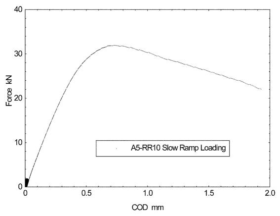
FIG. A15.1 Typical Force versus Displacement Curve
