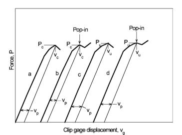
Note 1—Construction lines drawn parallel to the elastic loading slope to give  $v_p$ , the plastic component of total displacement,  $v_g$ . Note 2—In curves b and d, the behavior after pop-in is a function of machine/specimen compliance, instrument response, etc.
