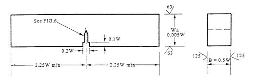
Note 1—The two side planes and the two edge planes shall be parallel and perpendicular as applicable to within  $0.5^{\circ}$ .
