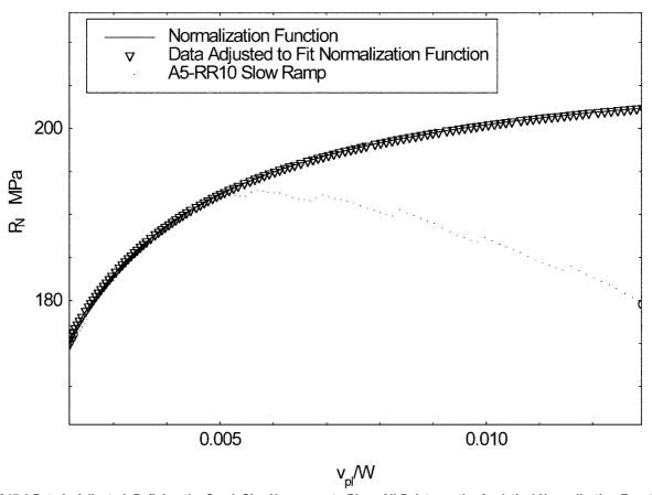
FIG. A15.4 Data is Adjusted, Defining the Crack Size Necessary to Place All Points on the Analytical Normalization Function (Only a portion of the data is shown for clarity)
