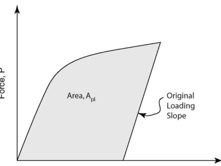
Total Load-line Displacement, v
