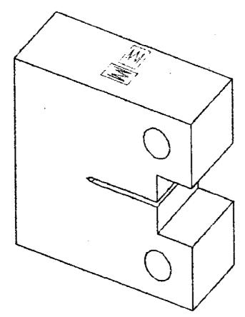
FIG. A14.2 Strain Gages Mounted on C(T) Specimen for Measurement of Transmitted Force
