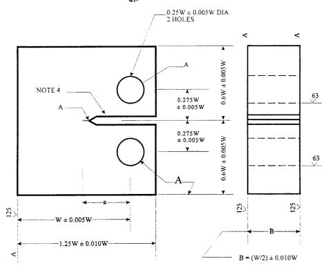
Note 1—A surfaces shall be perpendicular and parallel as applicable to within 0.002 W TIR.
