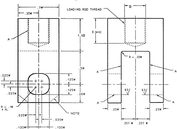
A - SURFACES MUST BE FLAT, IN-LINE AND PERPENDICULAR, AS APPLICABLE, TO WITHIN 0.002 in. T.I.R. (0.05 mm)
