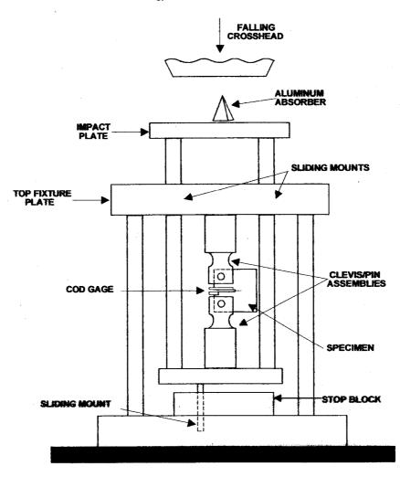
FIG. A14.4 Test Fixtures for Drop Tower C(T) Specimens
