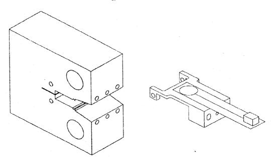
FIG. A14.5 High Rate Capacitance COD Gage and C(T) Specimen with Attachment Holes
