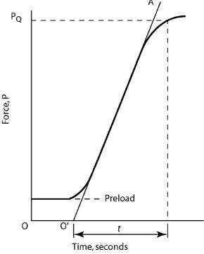
FIG. A13.2 Determination of Test Time from Force versus
