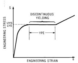
FIG. 1 Stress-Strain Diagram for Determination of Upper and Lower Yield Strengths and Yield Point Elongation in a Material Exhibiting Discontinuous Yielding
