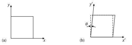
The shear strain is defined as  $\gamma = \tan \theta$ . The deformed axes can be described in terms of the original axes as,
