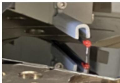
d. Check if the center of red stylus reticle matches with the tip of stylus
