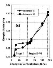
Fig. 7. Measured and Estimated Data on Section 400 of Phase I Structure: (a) Vertical Stresses, (b) Horizontal Stresses, and (c) Geogrid Strains.
