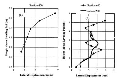
Fig. 8. Lateral Displacements Monitored on Phase I Structure: (a) during Stage I Construction, and (b) due to Placement of the Bridge Superstructure.
