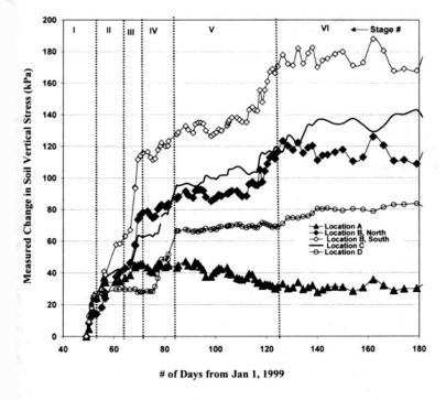
Fig. 10. Measured Vertical Soil Stresses during all Construction Stages (Measured between Geogrid Layers 10 and 11 along Section 800)
