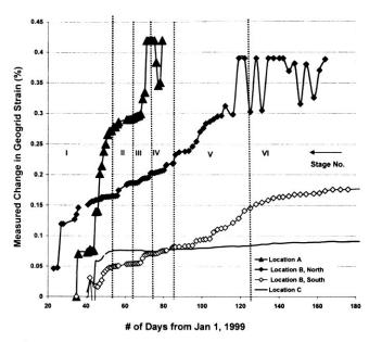
Fig. 11. Measured Geogrid Strains during all Construction Stages (Measured on the 6<sup>th</sup> geogrid layer of Section 800)
