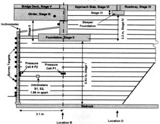
Fig. 6. Instrumented Section 400 indicating Construction Stages
