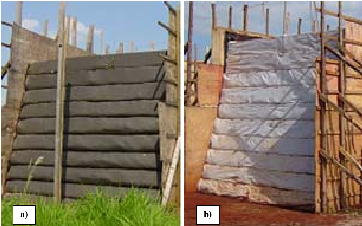
Figure 1. Front view of the prototypes: a) nonwoven geotextile (PET) and b) woven geotextile (PP).
