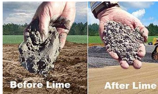
Figure 2.3.1: Increased friability in lime-treated clay (Carmeuse, 2018).
