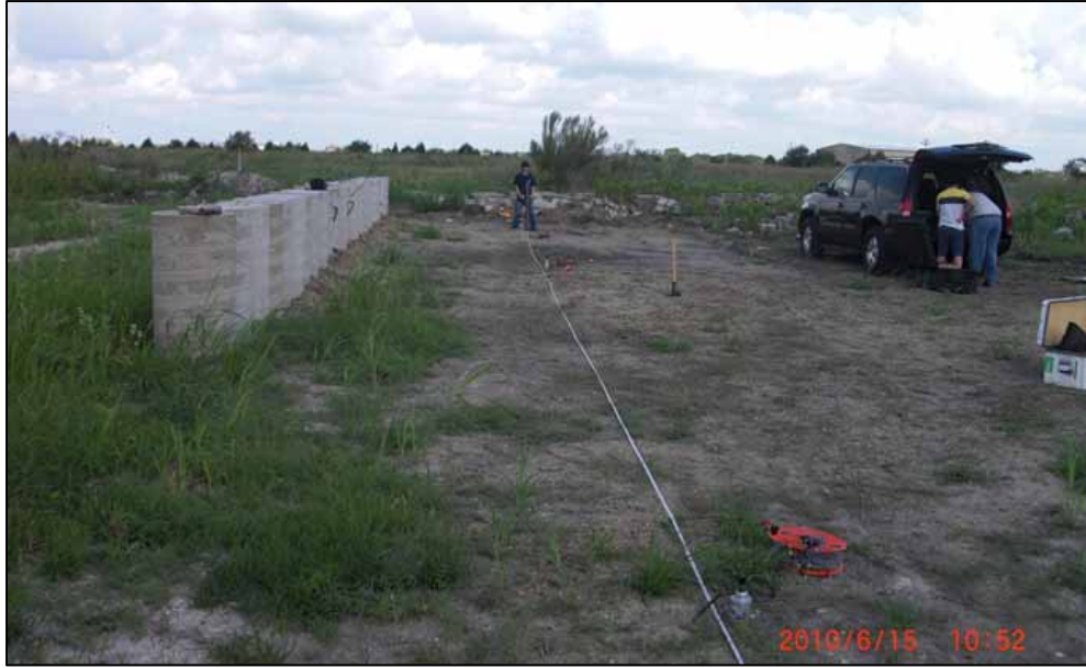
Figure 6.5: SASW testing at the test wall prior to excavation, June 2010.
