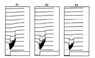
Figure 4. Failure mechanisms of the transverse sections of Model 2 (flexible pipe in dense backfill)
