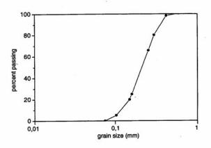
Figure 2. Grain size distribution of the sand used as backfill
