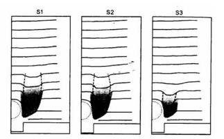
Figure 5. Failure mechanisms of the transverse sections of Model 3 (rigid pipe in loose backfill)
