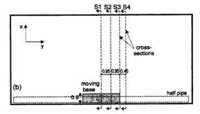
Figure 1. a) Scheme of model configuration; b) plan view of model showing positions of the transverse sections. Prototype dimensions (m)
