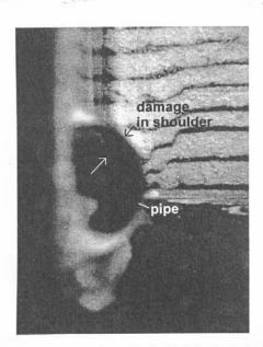
Figure 9. Damage experienced by the flexible pipe in the loose backfill (Section 1)
