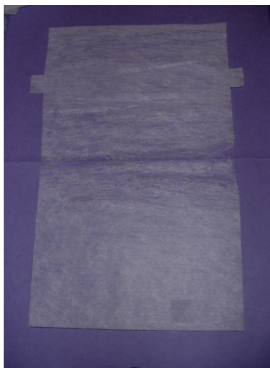
Fig. 12. View of geotextile reinforcement retrieved after failure of centrifuge model (Model F2, Layer 6).
