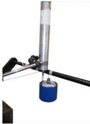
Figure 3. Displacement transducer and dead weight.
