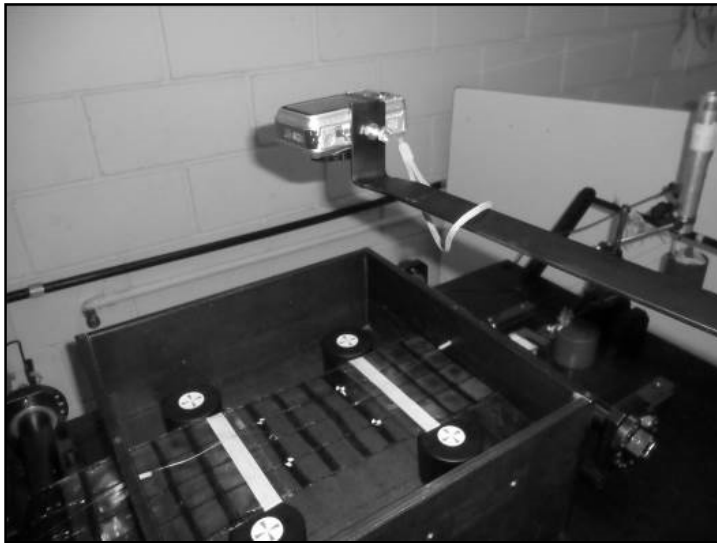
Figure 2. Data acquisition set with video camera, reference and on-specimen points.
