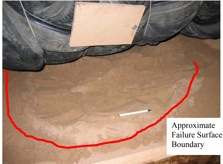
Figure 6.40: Approximate Failure Surface for the Tire Bale-Sand Interface for an Applied Normal Stress of 88 psf (Self Weight of Bale Only)
