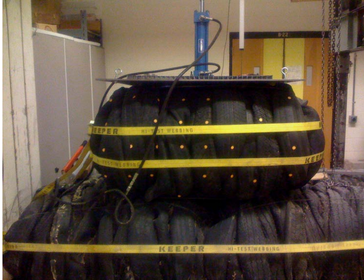
Figure 7.14: Placement of Nylon Cargo Straps Around the Mid-Section of the Tire Bales
