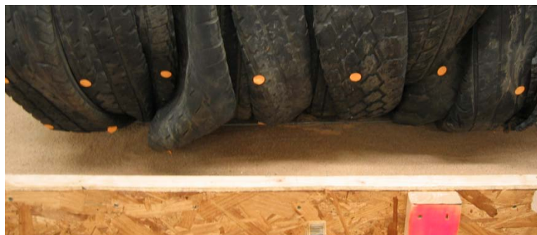
Figure 6.41: Photograph of the Rounded Bale Interface at the Tire Bale-Sand Interface Contact Area
