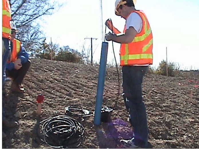
Figure 9.6: Taking Inclinometer Readings
