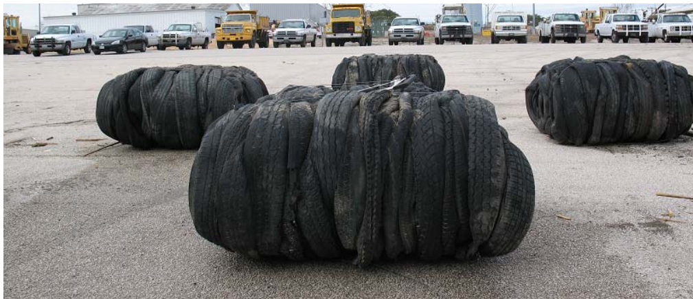
Figure 8.41: Photograph of Four Tire Bales at the TxDOT Facilities
