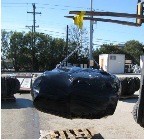
(a) Tire Bale Wrapped in Plastic.
