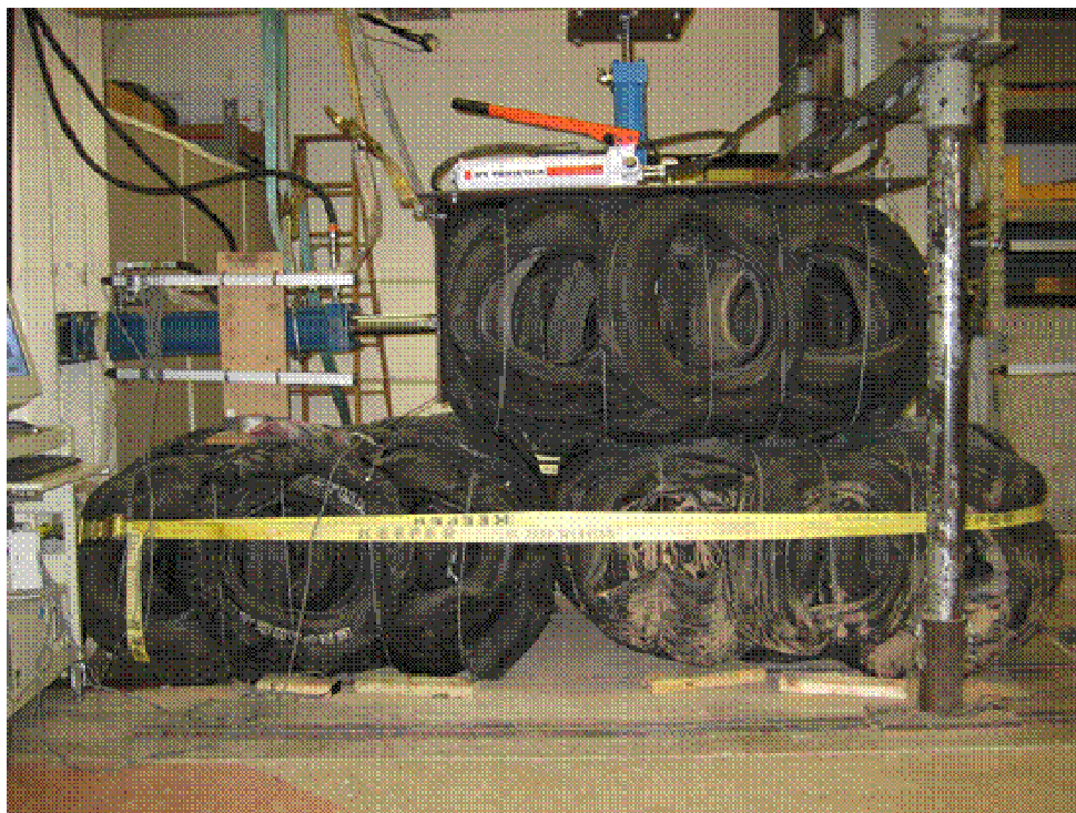
Figure 6.19: Anisotropic Tire Bale Direct Shear Testing Setup
