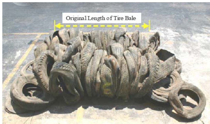
Figure 3.1: Rapid Expansion Testing of Tire Bales (LaRocque 2005)
