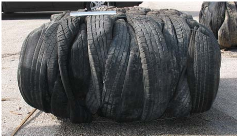
Figure 5.3: Photographs and Average Dimensions of the Five Tire Bales Used for the Index Testing Program
