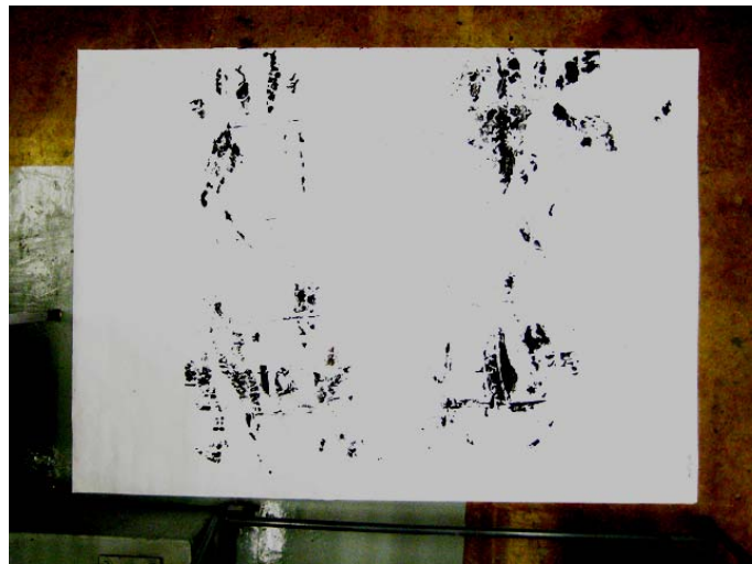
Figure 6.36: Photograph of a Tire Bale Interface Stamp
