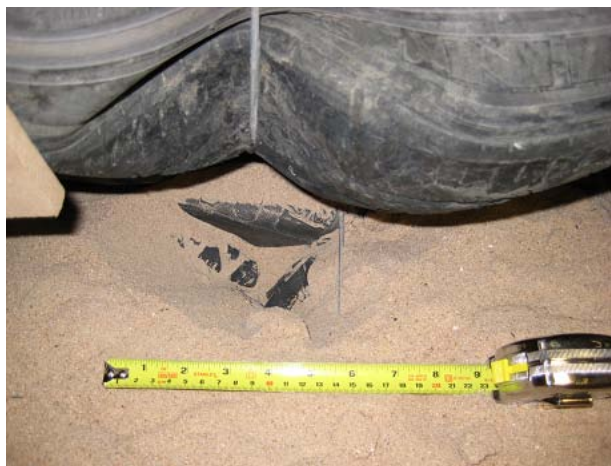
Figure 6.33: Sand Sink Holes Measured Along the Surface of the Thick Sand Interface
