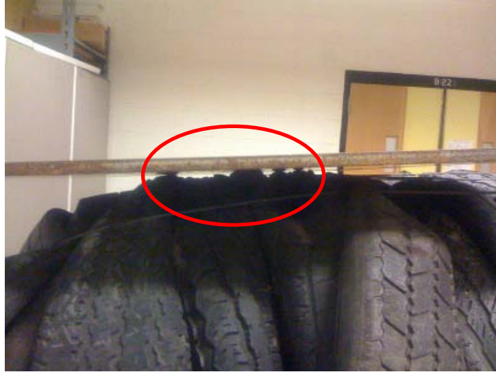
Figure 7.9: Photographs of the Contacts between the Rigid Top Plate and the Tire Bale for both Bale Arrangements
