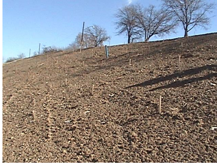
Figure 9.5: Location of Stakes Placed Along Slope Surface for Surveying
