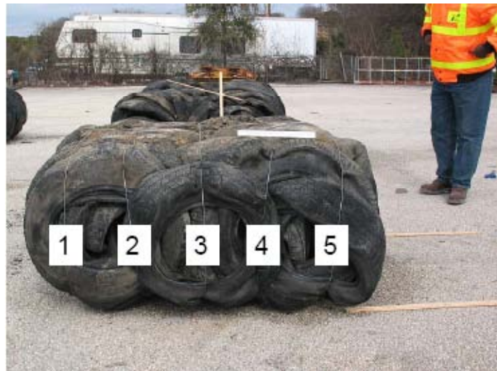
Figure 5.10: Tire Bale Wire Numbers and Rapid Expansion Test Setup
