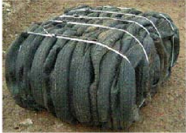
Figure 5.8: Placement of Extra Geosynthetic Straps around a Tire Bale with Galvanized Steel Baling Wires (www.angloenvironmental.com)
