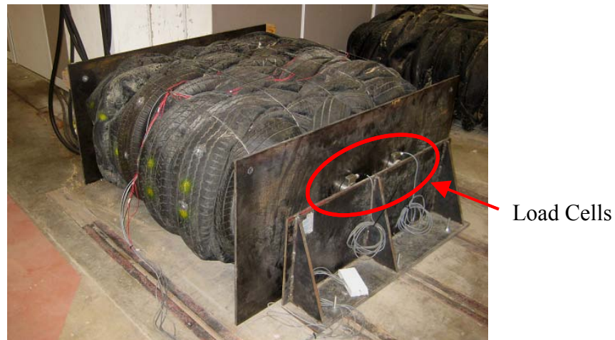
Figure 5.13: Photograph of the Horizontal Pressure Testing Setup
