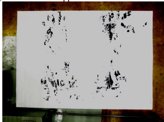
Figure 11. Digital Photograph of a Tire Bale Interface Stamp.
