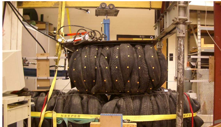
Figure 2. The Large Scale Direct Shear Test Setup for Tire Bales.
