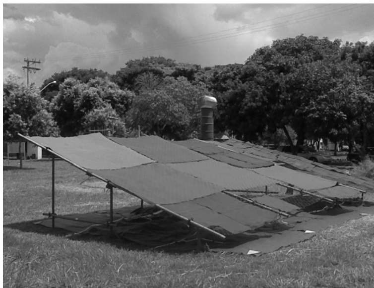
Figure 1. PET non-woven geotextile samples exposed to weathering
