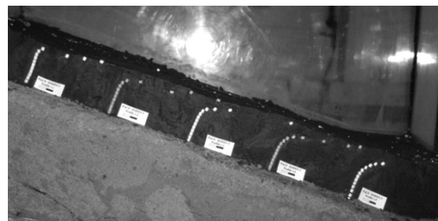
Figure 3.29. Soil movement shown by markers after 1 thawing cycle of thawing (Harris et al. 2008).
