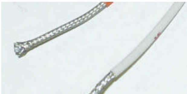
Figure 3.9. TDR cables: 0.59 mm diameter 75 Ω (left), 1.02 mm diameter 50 Ω (right) (McAlister & Pierce 2001).
