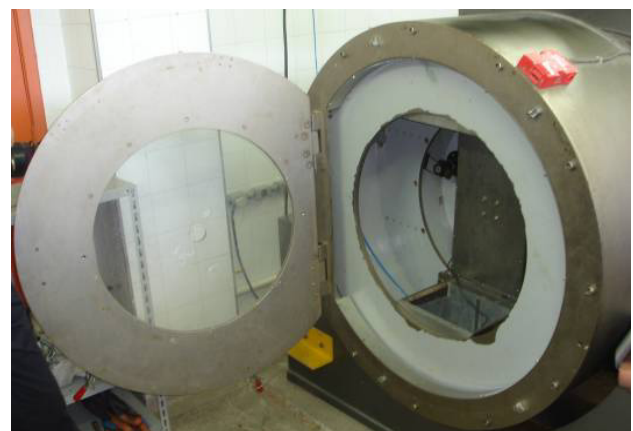
Figure 3.8. Drum centrifuge rotated on horizontal axis in soil preparation mode at COPPE, Rio de Janeiro (Photo: Springman).
