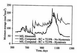
Figure 10: Effect of including hysteresis in the soil water characteristic curves
