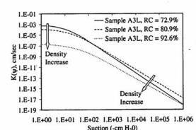
Figure 2: van Genuchten-Mualem unsaturated hydraulic conductivity functions
