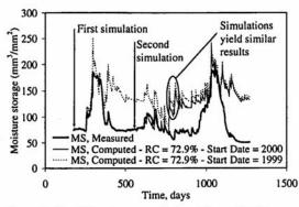
Figure 7: Variation in computed moisture storage for two different model starting dates
