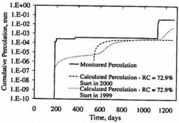
Figure 11: Comparison between monitored and computed basal percolation
