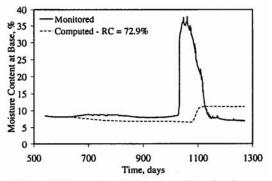
Figure 6: Comparison between monitored and computed basal volumetric moisture content
