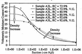
Figure 1: Suction-volumetric moisture content relationship for the cover soil
