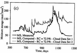
Figure 9: Sensitivity analysis to meteorological input parameters: (a) Solar radiation; (b) Wind speed; (c) Percent Cloud Cover
