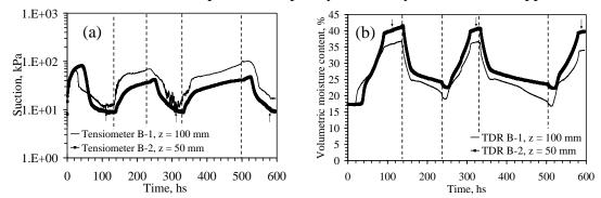
Figure 9: Profile B: (a) Suction; (b) Moisture content (Arrows denote breakthrough)
