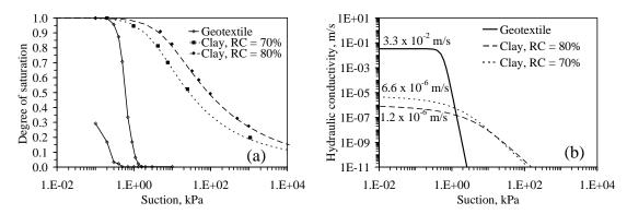
Figure 1: Hydraulic properties of compacted clay and nonwoven geotextile; (a) Water retention curves; (b) K-functions predicted from WCRs
