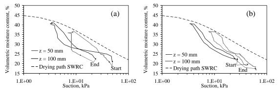
Figure 10: Transient WRC for Profile B: (a) Cycle 1; (b) Cycle 2
