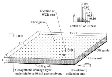
Figure 2: Schematic of the landfill test cover
