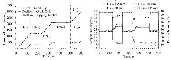
Figure 8: (a) Cumulative inflow and outflow; (b) Temperature and relative humidity
