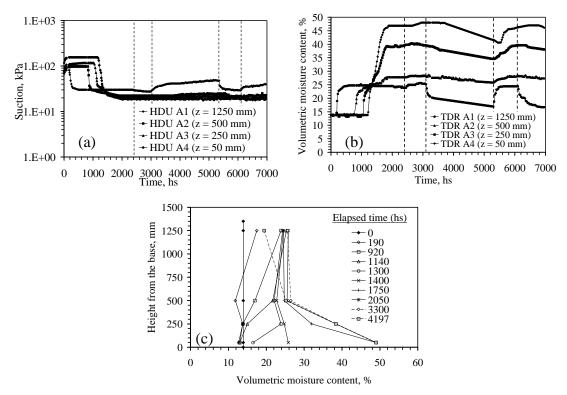
Figure 7: Profile A: (a) Suction; (b) Moisture content; (c) Moisture content profiles
