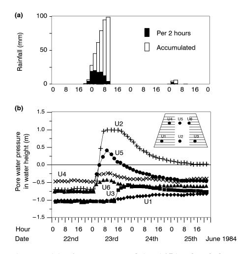
Figure 6. Variation of pore water pressures during rainfall in a clay embankment reinforced with nonwoven geotextiles: (a) rainfall recorded; (b) pore water pressures (after Tatsuoka and Yamauchi 1986).
