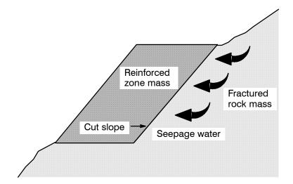
Figure 17. Water infiltration in a reinforced slope for road widening projects.
