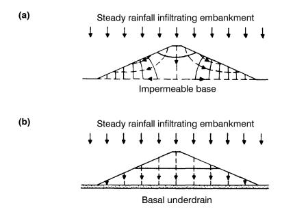
Figure 18. Flow regime for embankment: (a) on an impermeable base; (b) on a pervious base (after Ingold 1992).
