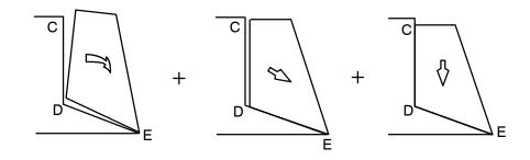
(a) Rotation about the toe (b) Sliding along DE (c) Settlement due to local compression failure at the toe
