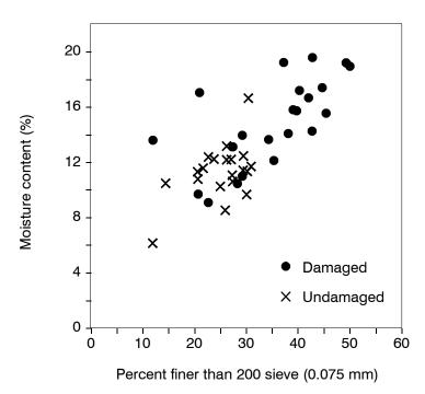
Figure 8. Moisture content and percentage fines for damaged and undamaged walls reinforced with metallic strips (after Elias and Swanson 1983).
