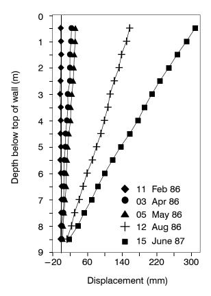
Figure 10. Horizontal displacements versus depth recorded at a geogrid reinforced wall (after Burwash and Frost 1991).
