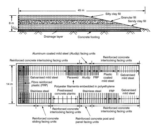
Figure 1. Transport and Road Research Laboratory (TRRL) experimental reinforced wall (after Boden et al. 1978).
