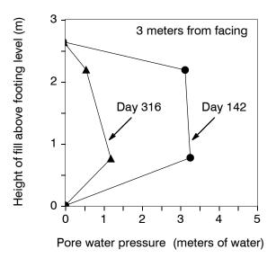
Figure 2. Vertical distribution of pore water pressure in the lower cohesive layer of the TRRL experimental wall (after Murray and Boden 1979).
