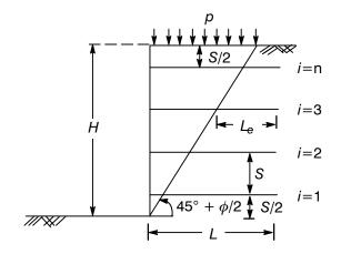
Figure 7. Arrangement of reinforcements in a clay wall model (after Ingold 1981).
