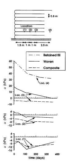
Figure 5. Pore water pressures (*u*) recorded in the Rouen reinforced wall, along a woven and a nonwoven/geogrid composite, at different locations within the silty backfill (redrawn after Perrier et al. 1986).
