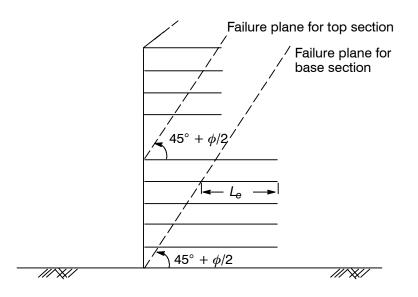
Figure 9. Configuration of welded wire wall on Interstate 580, California (after Mitchell and Villet 1987).
