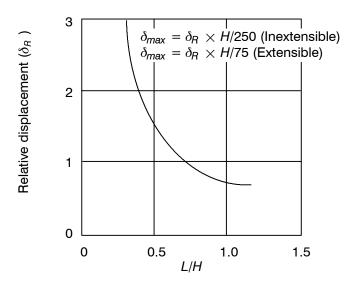
Figure 14. Curve for estimation of lateral displacement anticipated at the end of construction of reinforced walls (after Mitchell and Christopher 1990).
