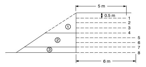
Figure 16. Geotextile reinforced wall on Autoroute A15, France (after Puig and Blivet 1973).
