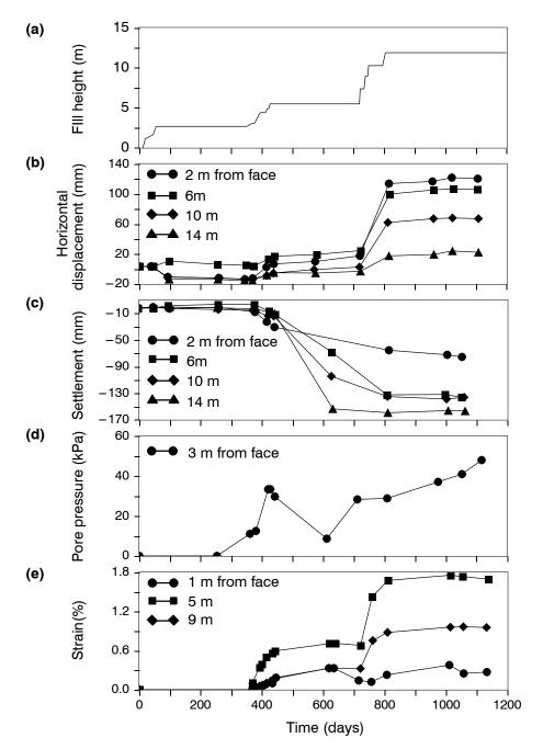
Figure 4. Field measurements at 3 m above base and at various distances from slope face within embankment and geogrids of Devon test fill: (a) fill height; (b) horizontal displacements; (c) settlements; (d) pore pressures; (e) geogrid strains (after Sego et al. 1990).
