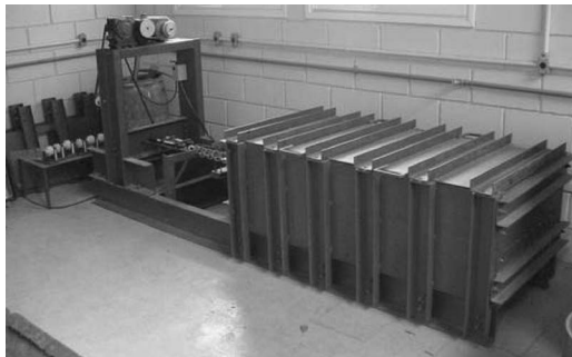
Fig. 2. View of large-scale pullout test device used in this study
